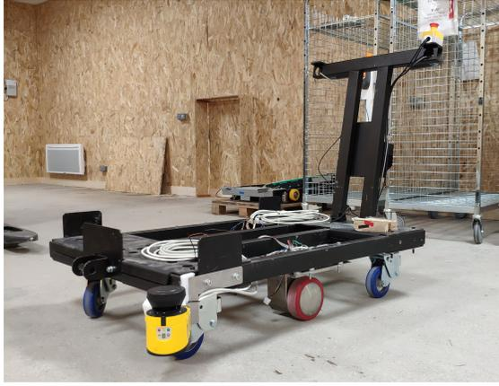
Fig. 6. The first prototype of our *SmartTrolley* experimental mobile platform, in the test room.
